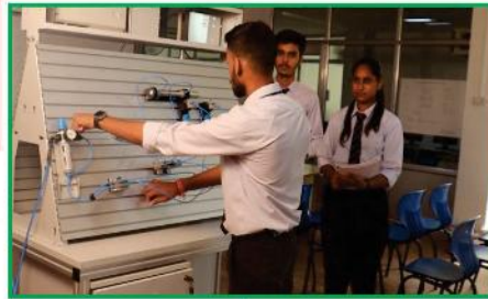
Students preparing pneumatic circuits on Didactic setup by Festo India
